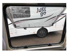
2 The windows work on a ratchet system so you need to make sure that you open it to the desired level and click in place.
