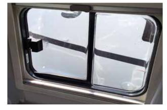
Simply hold and release the trigger on the window catch and slide the window to the right. To close pull the window back to the left and click the catch back into place.
