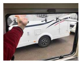
When you want to close the window, simply push the window up to it's fullest extent to allow it to fall back down to a closing position. Click the handles back in place to secure.
